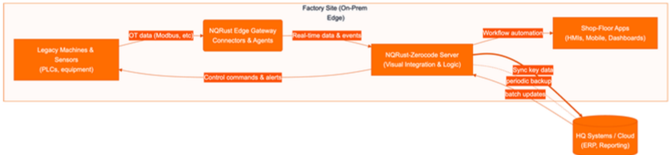
Figure 4: Solution 1 Architecture – A local NQRust-powered edge hub connects factory machines, workers, and HQ systems.
